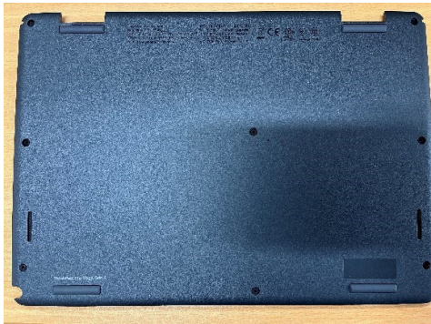
Bottom cover: used to hold the internal components and is attached to the palm rest.
