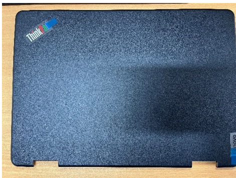
Top cover: used as the main part of the lid and is used to clip the screen in place.
