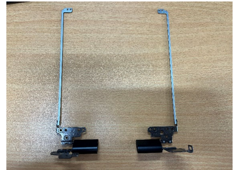
Hinges: used to connect the whole top of the notebook to the bottom of the notebook
