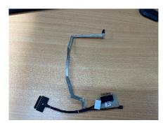
EDP cable: Used to connect the screen to the internals of the notebook for it to show a display.
