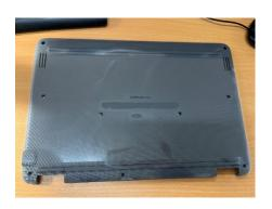
Bottom cover: used to hold the internal components and is attached to the palm rest.
