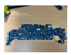
Motherboard: is the main internal part of the notebook that is used to provide connections to the other parts of the notebook
