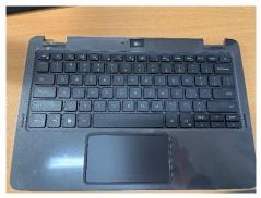
Palm rest keyboard: attached is keyboard and trackpad.
